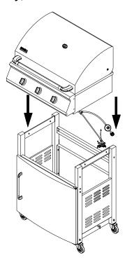
Step9: Open the lid, take out the cooking grid first, then screw tighten the four (4) pcs of 1/4\*12 screws into the left side and right side of firebox as shown figure below.
