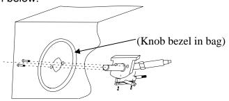
Step 8: Place knob on valve stem, then screw the knob by using the wrench tool.
