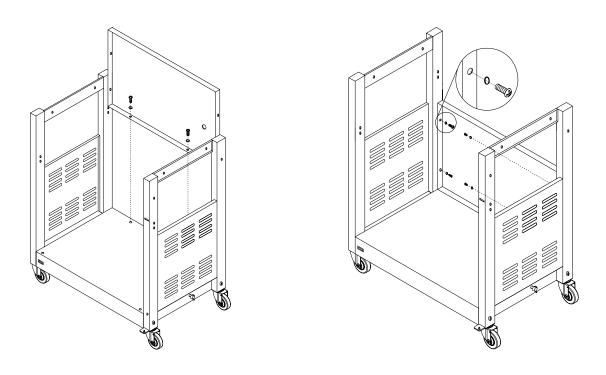
Step 4: Assemble the front cart and back cart frame to the front side and back side of the side panel with eight (8) pcs of screws.
