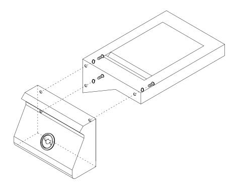
Step12: Assemble side shelf and side burner with eight (8) pcs of 1/4\*12mm screws as figure shown below.
