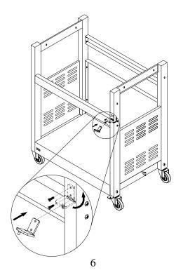
Step 6: Assemble the door on the hinge bracket from bottom and tighten the screws on top hinge bracket.
