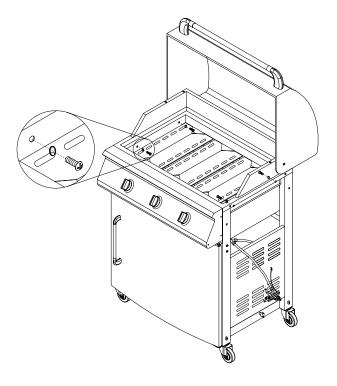
Step10: Assemble side shelf front panel to the left side shelf with two (2) pcs of 1/4\*12 mm screws as the figure shown below.
