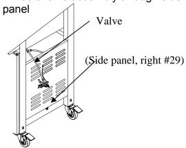
Step 2: Remove 4(four) screws & washers from the "U" brackets on the side
