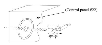
Step 6: Align & tighten knob bezel & valve stem with 2(two) screws & washers as shown below.
