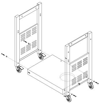
Step 3: Assemble the back panel to the two side panels with two (2) pcs of 1/4\*12 mm screws and four (4) pcs of 5/32\*10mm screws as shown figure below.
