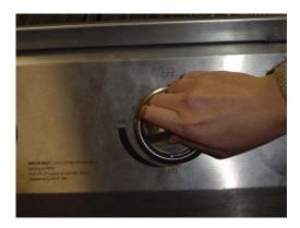
Step2. Push and turn one of main or side burner knobs to HI position
