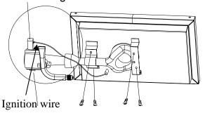
Step 4: Insert valve stem assembly through knob hole to the control panel
