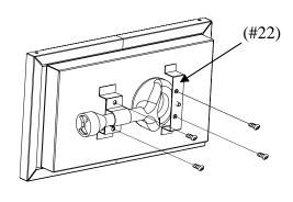
Step 3: Insert valve stem assembly into burner venturi
