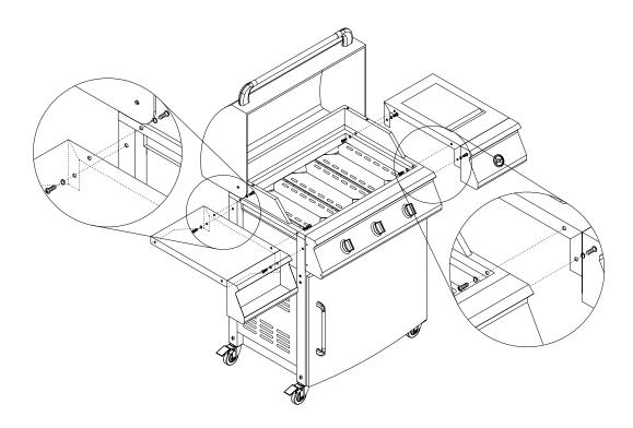
Step13: Insert spice tray and side burner control panel into control panel with two (2) pcs of 5/32\*10 mm screw, and as figure shown below.
