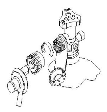
**CAUTION!** ASSEMBLY TO PROPANE TANK .DO NOT USE TOOLS TO ATTACH REGULATOR /HOSE ASSEMBLY TO PROPANE TANK.
