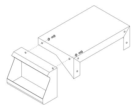
Step11: Assemble the control panel to the side burner with three (3) pcs of 1/4\*12mm screws as figure shown below.
