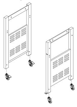
Step 2: Assemble bottom panel to side panels with four (4) pcs of 1/4\*42 mm screws as shown figure below.
